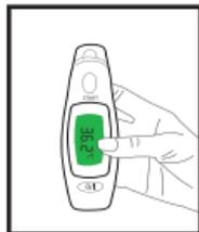
5. Press the **START** button once and release it. Start to move the instrument steadily from 1 cm above the center of the eyebrow to the temple area. A long beep sound will emit after 3 seconds to acknowledge the completion of measurement. If the probe movement is too slow to reach the temple area before the long beep sound is heard, repeat the measurement as described above, but simply move the probe a little quicker this time.
